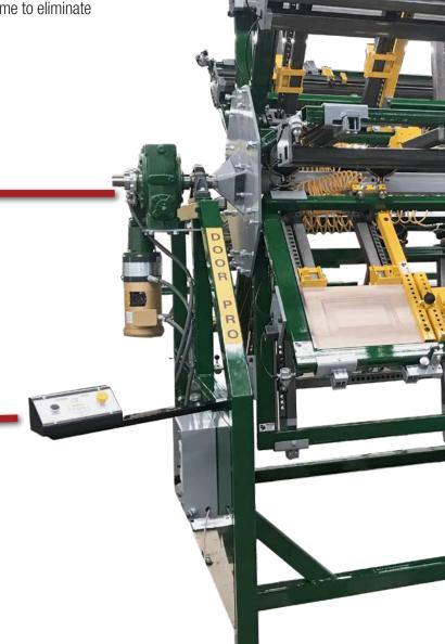
In a typical door shop glue is applied and components assembled on an assembly table. The door is placed in a section and clamps adjusted. The cylinders are activated by one vale which first creates side pressure pushing the door on the left side square, a second later the vertical clamps are activated to create pressure on the glue joints.
