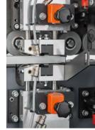
Surface scraper with dual-tracing
